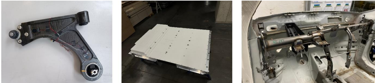
Figure 1 LEVIS Demonstrators (from left to right: suspension control arm, battery holding set, cross car beam)
