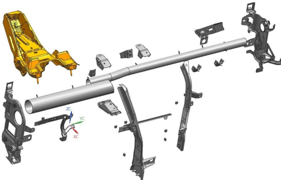
Figure 53: Visual representation of the cross car beam. Golden part (steering column carrier) is part of the LEVIS project.
